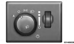
To turn on the headlights, rotate the headlight switch clockwise. When the headlight switch is on the parking lights, taillights, license plate light and instrument panel lights are also turned on. To turn off the headlights, rotate the headlight switch back to the O (Off) position.
